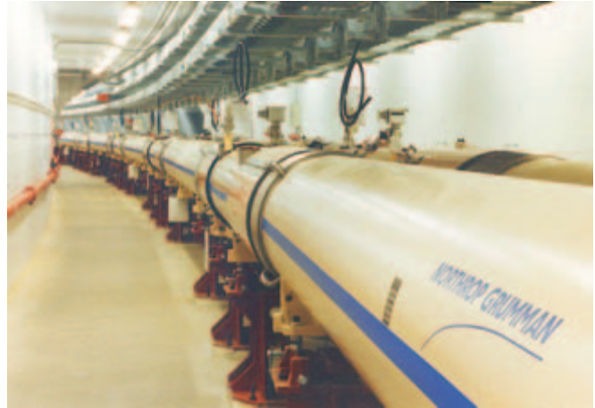
Relativistic Heavy Ion Collider (RHIC) at Brookhaven National Laboratory. The machine itself is enclosed in a tunnel, 12 feet under the ground. Inside two tubes, ion bunches race around RHIC's 2.4-mile ring in opposite directions.
