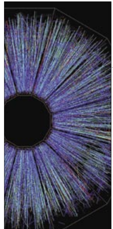
End view of a collision of two 30-billion-electron-volt gold beams in the Solenoidal Tracker at the Relativistic Heavy Ion Collider (STAR) at BNL. The beams travel in opposite directions at nearly the speed of light before colliding.
