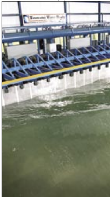
The tsunami wave basin at Oregon State University is the world's largest and most comprehensive shared-use research facility for the study of effects of tsunami inundation and storm waves on coastal buildings and lifeline infrastructures.
