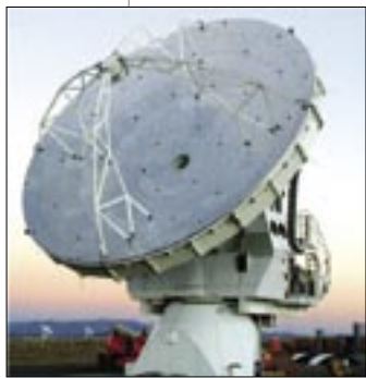
The ALMA VertexRSI test antenna, one of two prototypes constructed at the site of the Very Large Array near Socorro, NM.
