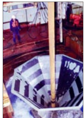
A re-entry cone, used to re-enter an existing drill hole on the ocean floor, starts its journey to the seafloor from the deck of the drillship JOIDES Resolution .
