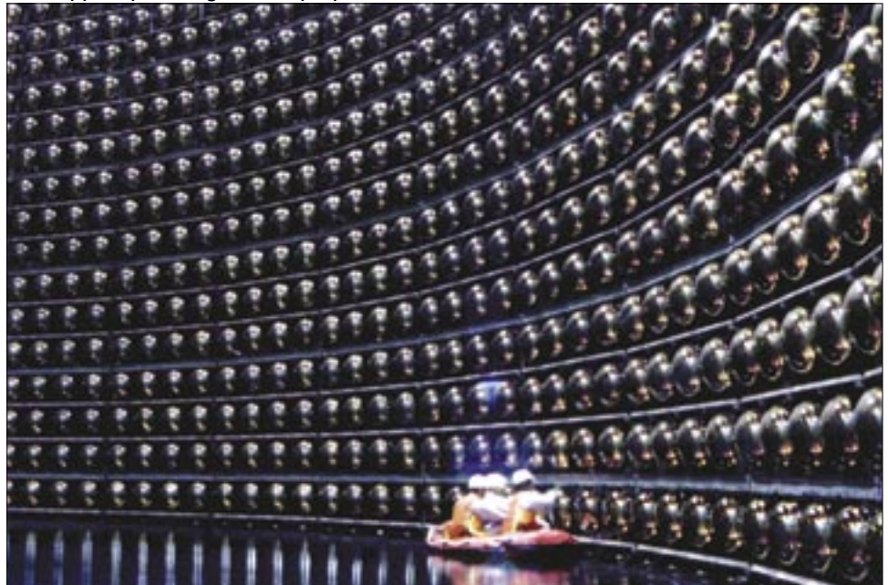
Located 2,000 feet underground in the Japanese Alps, the SuperKamiokande neutrino detector is composed of thousands of PM tubes, which collect light produced by the interaction of the neutrinos and the ultra-pure water filling the detector. This device has detected neutrino oscillations among atmospherically generated neutrinos, providing evidence that neutrinos have a small but finite mass. It has also detected solar neutrinos, contributing to the understanding of the problematic detection rate of neutrinos from the Sun.
