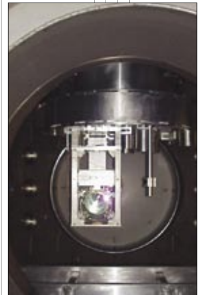
The End Test Mass in the x-arm of the 2k-IFO. (Hanford, WA)
