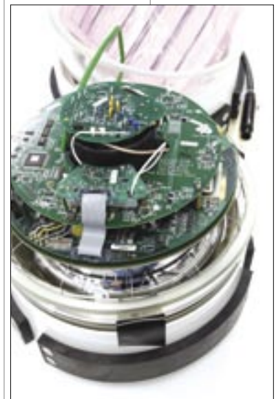
Pictured in the University of Wisconsin-Madison Physical Sciences Laboratory before being vacuum-sealed, each IceCube digital optical module or DOM is very much like a small computer. A total of 4,200 DOMs, designed to sample high-energy neutrino particles from deep space, are being deployed in 70 deep holes in the Antarctic ice. (November 2004)
