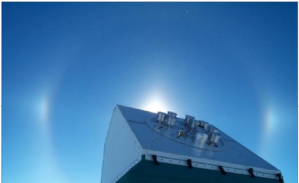
The Degree Angular Scale Interferometer (DASI), shown here, operates from the Amundsen-Scott South Pole Station is designed to measure temperature and polarization anisotropy of the cosmic microwave background radiation over a large range of scales with high sensitivity.
