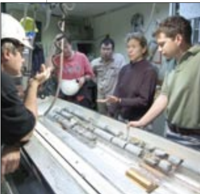
Scientists examine and discuss deep-sea rock cores on an Integrated Ocean Drilling Program expedition to the western rift flank of the mid-Atlantic Ridge.
