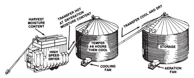
Figure 4. Schematic of dryeration system.
