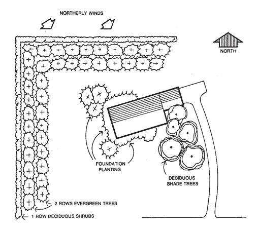
Figure 6. Recommended placement of shelterbelt for a farmstead.
