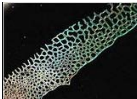
Not a snakeskin, but a magnified image of a dried polymer "ring" taken with an optical microscope. Credit: University of Massachusetts-Amherst.
