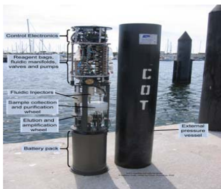
Genosensor used to detect pathogens in ocean and coastal waters. Credit: Image Courtesy of John Paul, USF.
