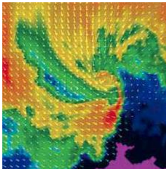
A simulation using the tornado detection algorithm. The swirling flow in the right-center of the image shows the tornado. Credit: CASA ERC, University of Massachusetts-Amherst.
