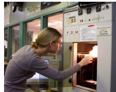
Mechanical engineering student creating a product prototype on a rapid prototyping machine in the Learning Factory. Credit: John Lamancusa, Penn State University.
