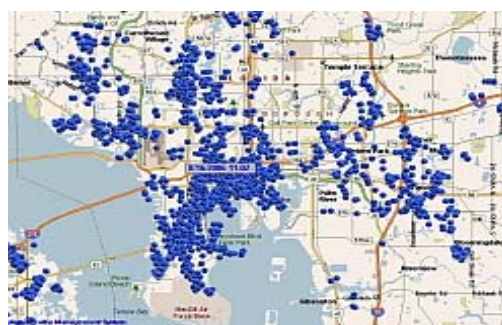
The IntelliOne Roadway Speed Measurement System uses cell phone signals to map roadway speeds for all highways and surface streets where mobile phone coverage exists. The blue dots represent a snapshot of all active mobile phones from a single carrier's network in Tampa, Fla. Credit: IntelliOne Technologies Corporation.
