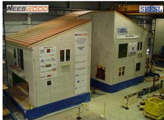
Full-size, two-story townhouse astride the NEES dual shake tables at the University at Buffalo, SUNY. Credit: John W. van de Lindt and the project web site http://www.engr.colostate.edu/NEESWood
