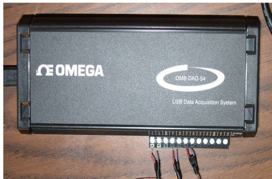
Fig. 19: Omega data acquisition unit (OMB-DAQ-54) used to acquire temperature readings throughout the mock wall section. Type E thermal couples were used in conjunction with this unit with measurements taken every 7.5 seconds. The thermal couple terminals are located at the bottom right of the unit. (Photo by author, 2007)
