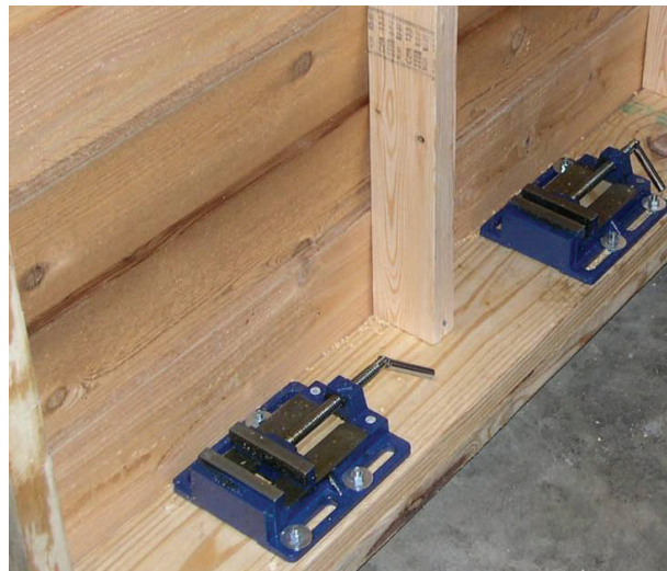
Fig. 28: Photo showing the clamps used to secure sample studs in the large mock wall section. Due to adjustability various sized wood members could be used. (Photograph by author, 2007)
