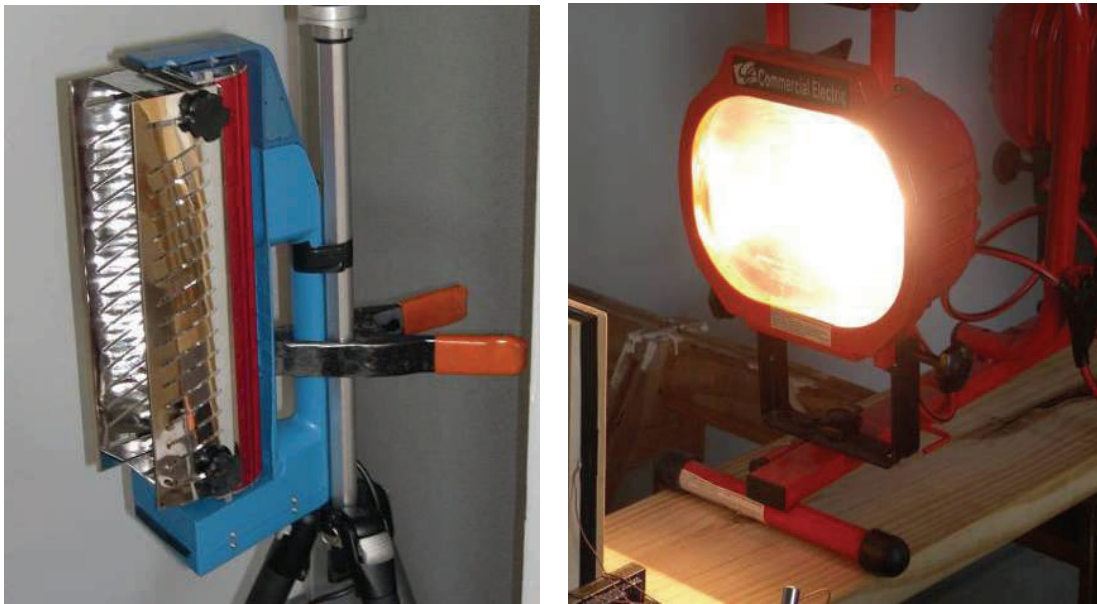
Fig. 21-22: Photographs showing the IR heat lamp on the left and the 300 watt type J lamp on the right. While the IR lamp posed a fire hazard the 300 watt lamp was able to be left unattended as temperatures never approached the threshold for thermal degradation. (Photo by author, 2007)
