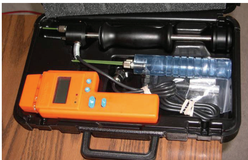
Fig. 20: Picture of the Delmhorst BD-2100 unit (orange) and accompanying pin set. The pin in the middle is used for deep wood penetration and is insulated on all sides so that the reading obtained is only from the tips of the pins. (Photo by author, 2007)
