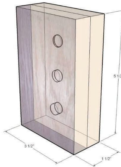
Fig. 33: Illustration showing the size of the wood sample used for deterioration analysis. Note the drilled holes. From top to bottom in terms of below surface depth/depth of simulated deterioration; 0.50”/0.25”, 0.63”/0.13”, 0.69”/0.06”. (Illustration by author, 2007)
