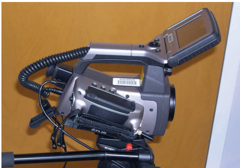
Fig. 16: Photo showing the ThermaCAM S65 HS mounted on a tripod for stationary viewing. Note the LCD screen for easy viewing and the straps for portability in the field. (Photo by author, 2007)
