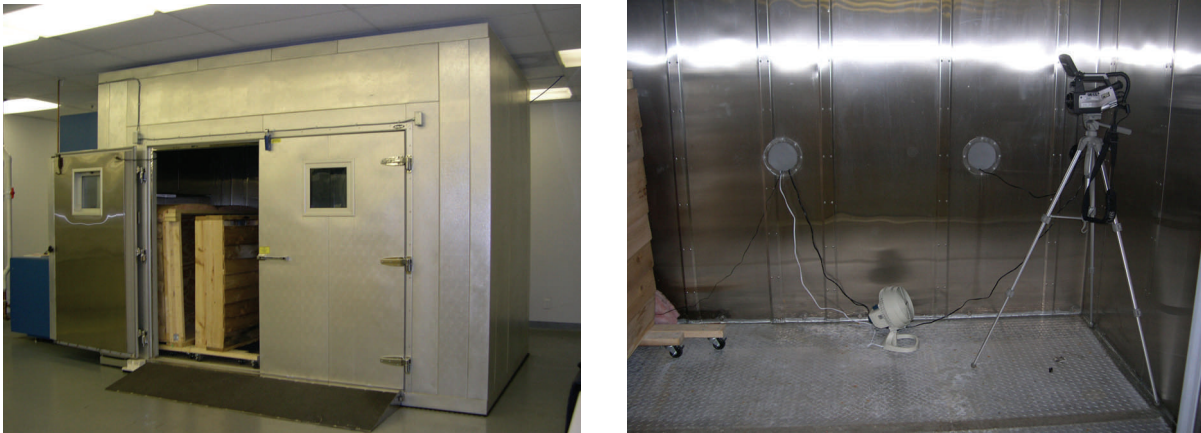
Fig. 30 & 31: Two images showing the environmental chamber at ESSC, Cincinnati, Ohio, used for testing the large wall sections. The two doors and ramp (left image) allowed the wall sections be we easily placed within the chamber. The interior of the chamber (right) shows the camera and the wall section (extreme left of the image). Note the wires passing out through the two holes (center), these connect the heating apparatus, thermocouples and IR camera to the computer outside the chamber. (Photo by author, 2007)
