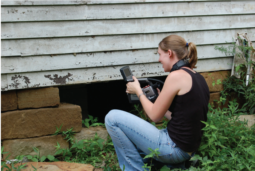
Fig. 51: Figure 51 shows University of Kentucky research assistant Laura Everdale using the IR camera to investigate a frame structure in Manchester, Kentucky. The IR camera helped provide information about the frame structure of the building as well as areas of moisture infiltration. (Photo by author, 2007)
