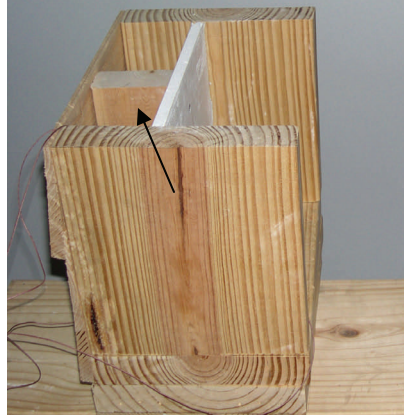
Fig. 23: Photograph showing one of the small 1'x1' wall sections. Clearly visible is the gypsum board (right), stud (arrow) and cedar siding (left). (Photo by author, 2008)
