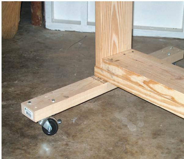
Fig. 27: Photo showing the casters used to wheel the larger wall sections into testing positions. The casters could also be locked to prevent sliding in transition or movement during testing. (Photograph by author, 2007)
