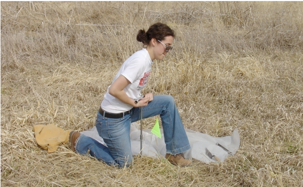
Figure 9. Coring with the JMC backsaver (above) and Oakfield push tube probe (below).
