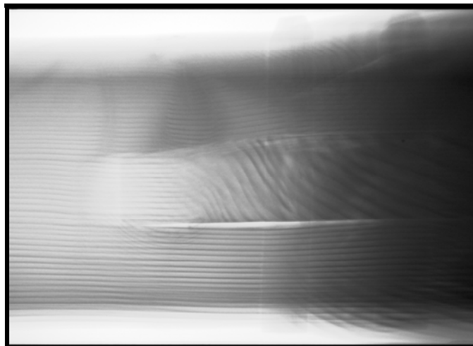
Figure 37. Radiograph of the mortise and tenon joint shown in Figure 36, as viewed from the back of the joint.
