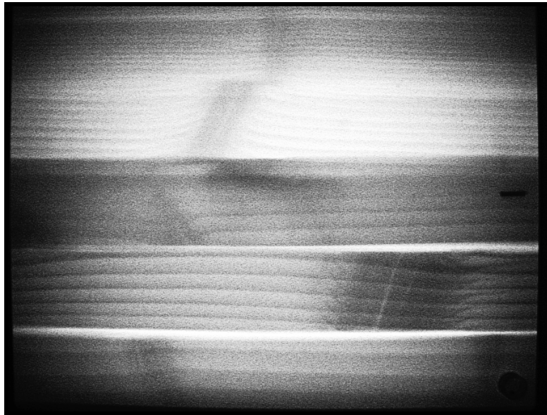
Figure 56. Modified radiograph of the wooden wall, using the histogram equalizer from the SAIC® imaging editing package.
