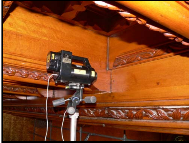
Figure 110. X-ray source positioned to take shot #15.
