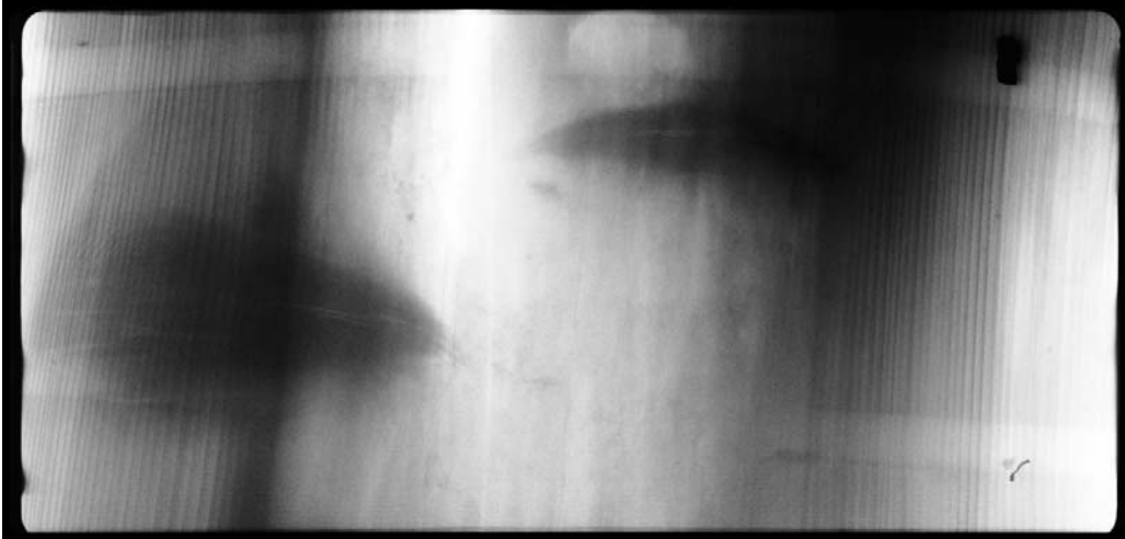
Figure 50. Radiograph of decayed log section.
