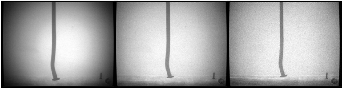
Figure 20. A six-inch thick block with embedded spike, x-rayed at 12, 24, and 36 inches between the source and the block, respectively. All radiographs have been adjusted for brightness and contrast to improve viewing in the report.
