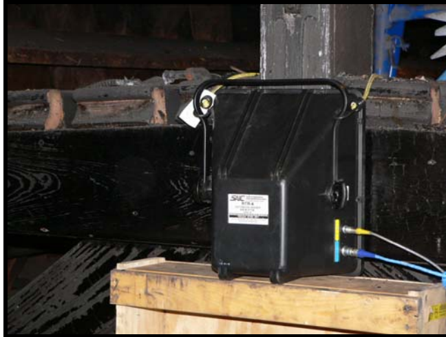
Figure 104. Imager placement for digital radiography at Location B2 on Truss 6.
