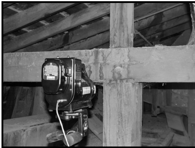
Figure 31. Mortise and tenon joint showing placement of x-ray source.
