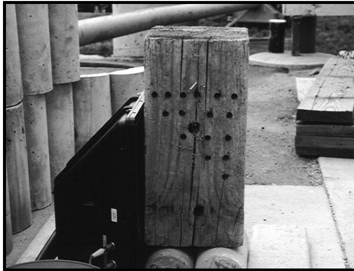
Figure 14. Simulated termite damage in timber.
