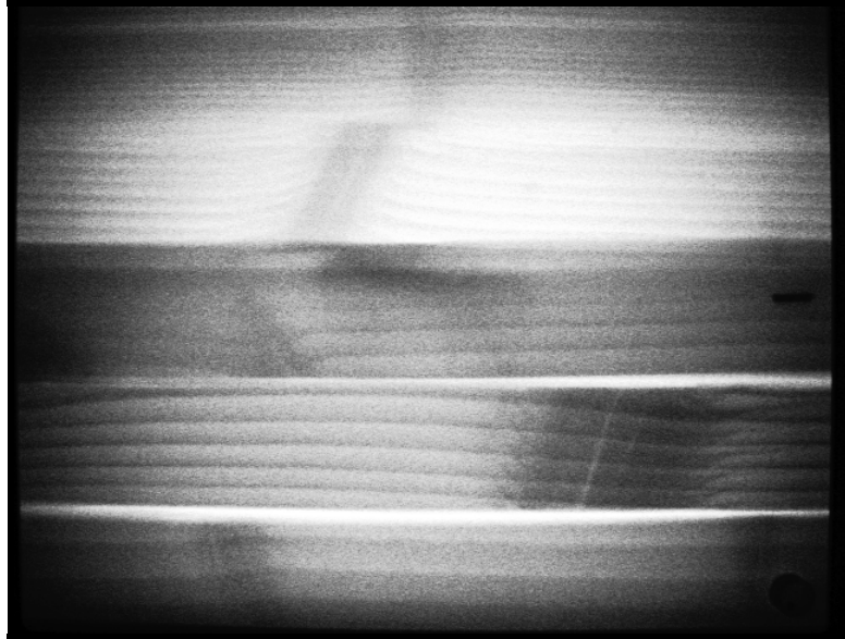
Figure 61. Modified radiograph of the wooden wall, using the equalize feature from the Logos Imaging software.
