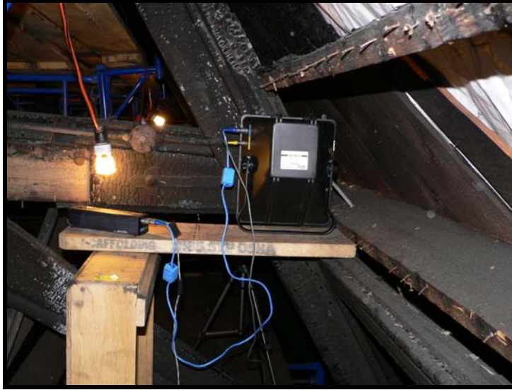
Figure 97. Imager placement for conducting digital radiosity for one setup at Location B1 on Truss 7 (north side).
