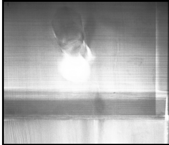
Figure 32. Radiograph showing peg and improperly drilled hole in the tenon.
