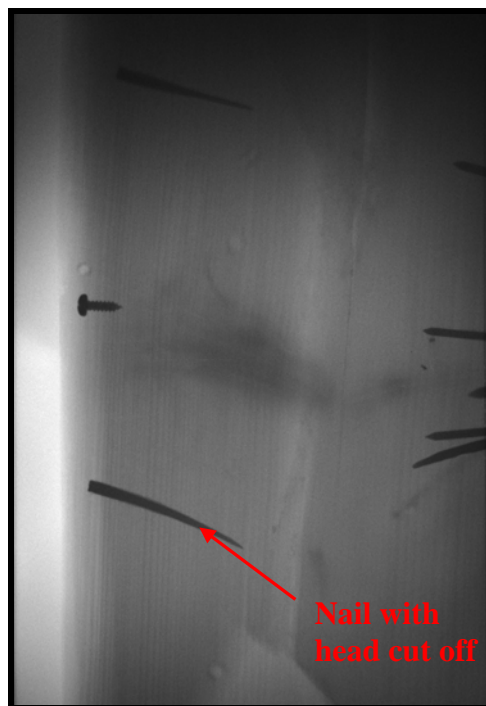
Figure 93. Radiograph showing a nail with the head removed.
