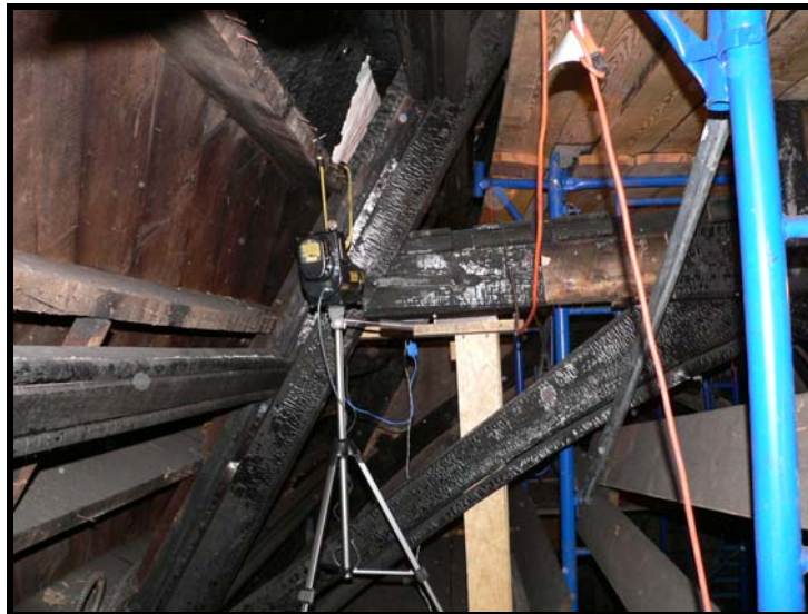
Figure 96. Source placement for conducting digital radiography for one setup at Location B1.
