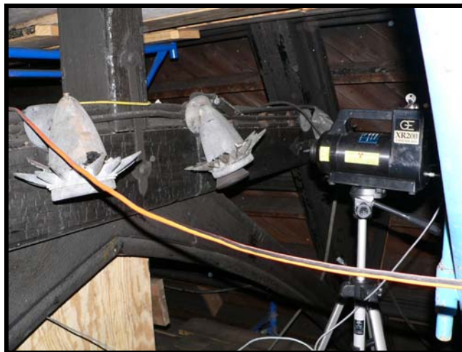
Figure 103. Source placement for digital radiography at Location B2 on Truss 6.
