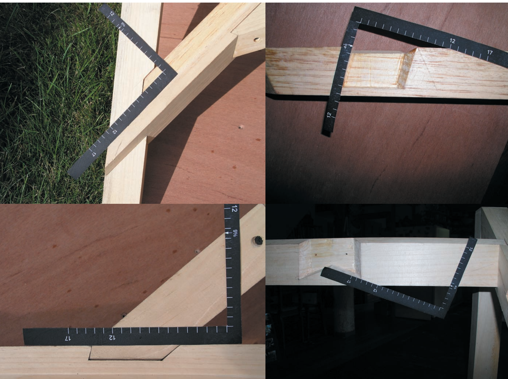
Model square laid over model joints to demonstrate layout of typical connections among valley, principal rafter, jack purlin, jack rafter and header (or ridge) in a valley dormer. Clockwise from upper left: valley rafter joint to principal rafter; jack purlin joint to valley rafter; seat cut for valley in header; and jack rafter joint to valley. Drawing of completed model and article, page 4.
