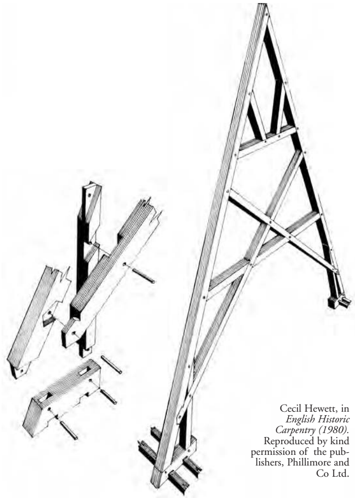
FIG. 2. SCISSOR-BRACED ROOF CROSS-FRAME, NORTHEAST TRANSEPT, LINCOLN CATHEDRAL, CA. 1200.
