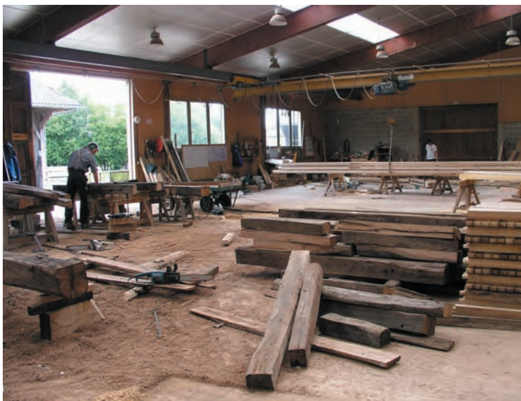
The workshop at Desperrois et fils. A rolling bridge crane and chain and circular saws make heavy work somewhat lighter. Most timber used is reclaimed, both for repair and new work.
