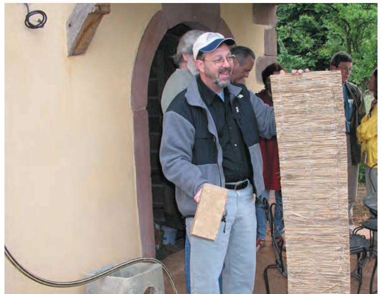
New Alsatian house in Ochfelden built in traditional style but using straw-clay brick infill and straw batt insulation, demoed below by a delighted Dave Carlon.
