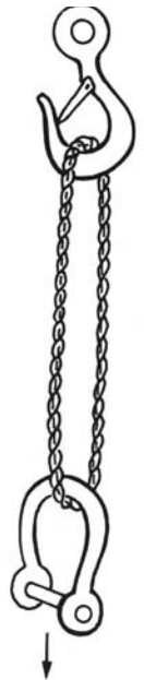
Vertical hitch, rope sling and shackle.
