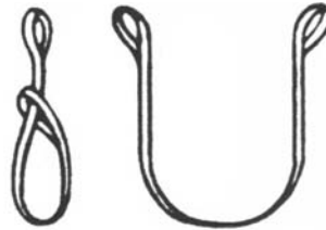
At left, eye-and-eye web straps shown in choker hitch (far left) and basket hitch.
