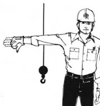
Boom down, cable up (flex fingers).
