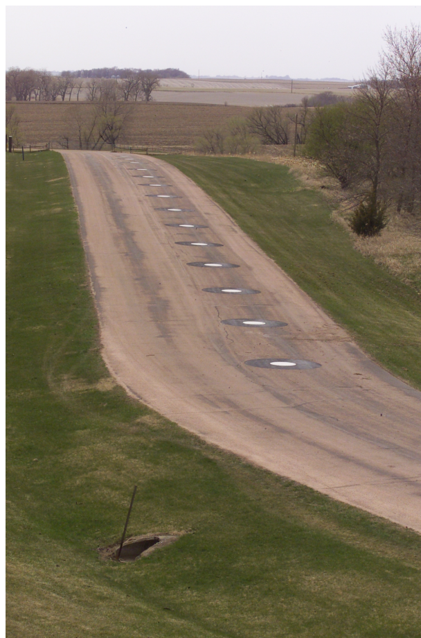
Figure 2. An example of calibration points in the Camera Calibration Range.
