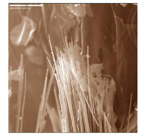
Scanning electron micrograph of asbestiform amphibole
