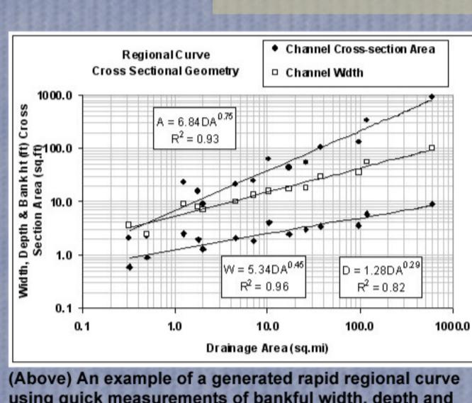
(Above) An example of a generated rapid regional curve using quick measurements of bankful width, depth and
