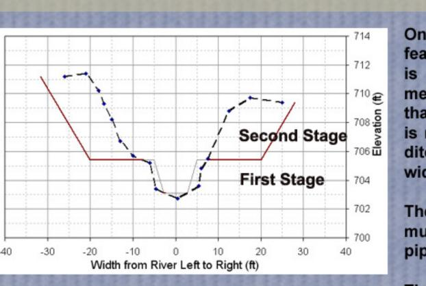
Once the bench feature is determined, the remaining design features of the channel can be designed. The pattern of the ditch is usually confined to the sinuosity of the ditch banks. Small that a "dog legged" stream will not functioning properly. Sinuosity is not part of a two stage design, however it is believed that the litch will determine its own sinuosity given adequate flood plain
