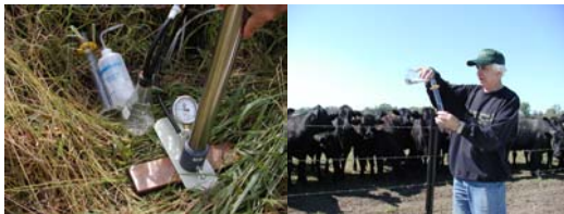
Figure 1. Soil solution sampling procedure: Vacuum at 55-65 kPa is applied to the suction-cup lysimeters; and Soil-water samples are collected after 18-24h
