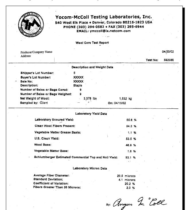
These Tests Performed According to ASTM D 584 and IWTO Method 12
