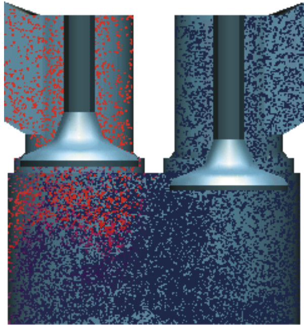
Fig. 3.1-1. A color visualization of the temperature field during the inlet flow in a hydrogen-fueled engine simulated with KIVA-3 [62][90]. The open intake valve is on the right; the closed exhaust port is on the left. The particles are used only to simulate the flow and are colored according to the temperature of the gas. The cold intake air (blue) is shown compressing the residual hot combustion gases (red).
