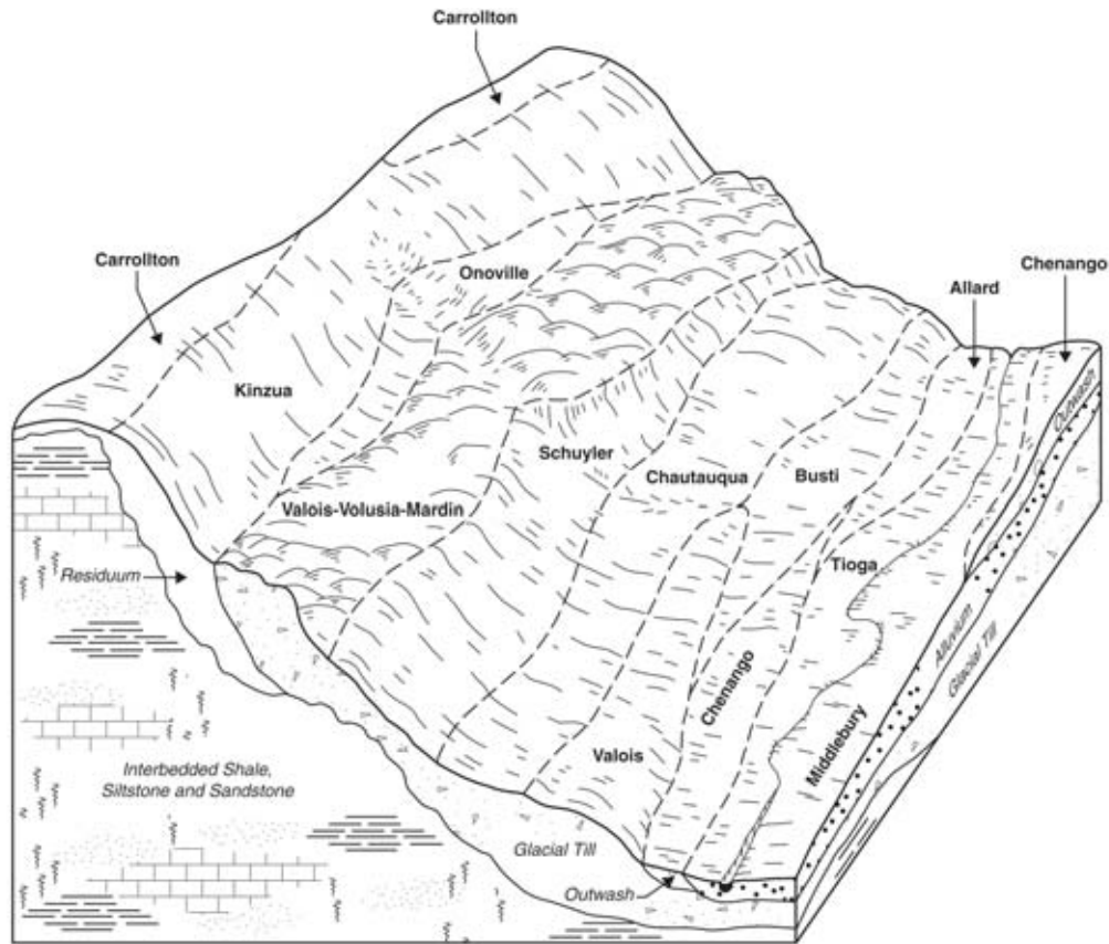
Figure 19.—Representative landscape showing soils that formed in residual material, glacial till, glacial outwash, or alluvium.
