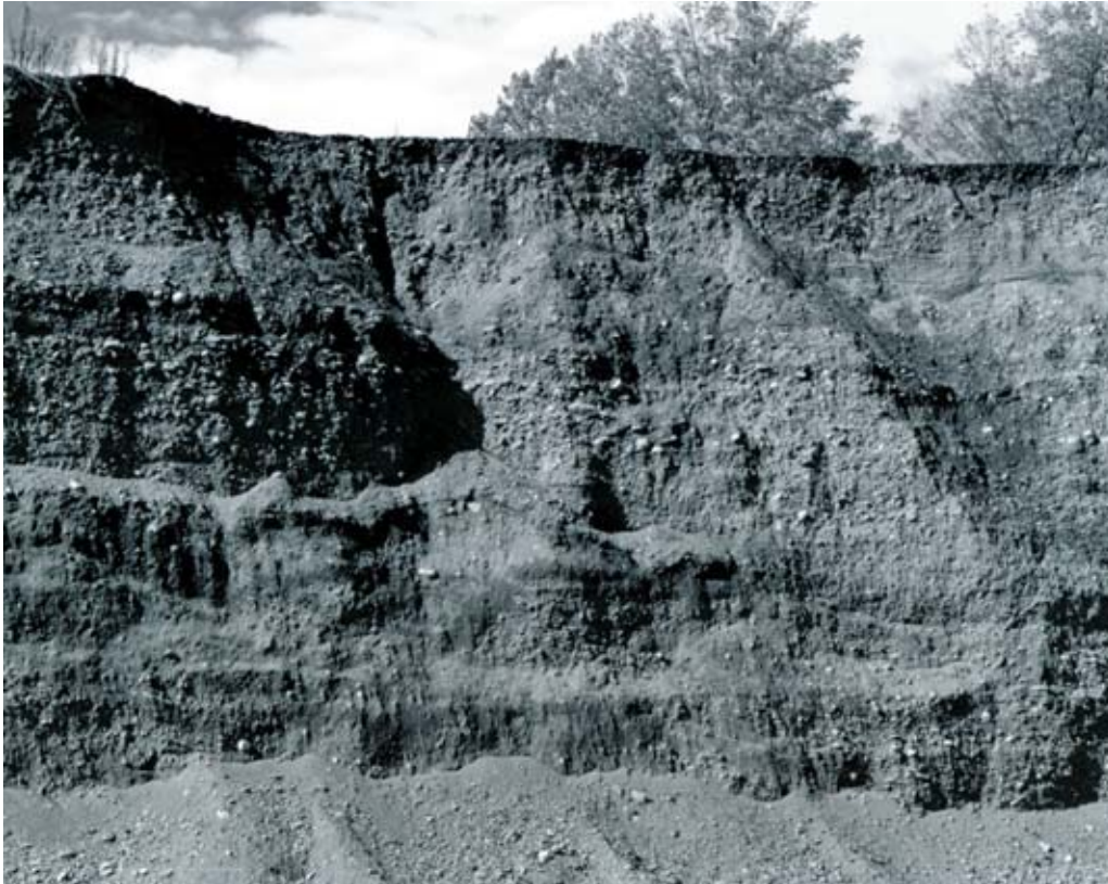
Figure 16. —Stratified glacial outwash deposit showing the variable layers of deposition. These gravelly deposits are a good source of sand and gravel.
