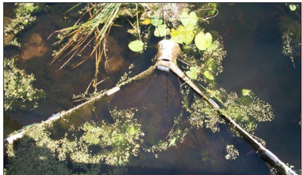
Figure 15. A small fyke net such as this one can be used to sample for juvenile fish as well as macroinvertebrates. Larger versions are also available for sampling larger, adult fish. Photo courtesy of Doug Wilcox, US Geological Survey.
