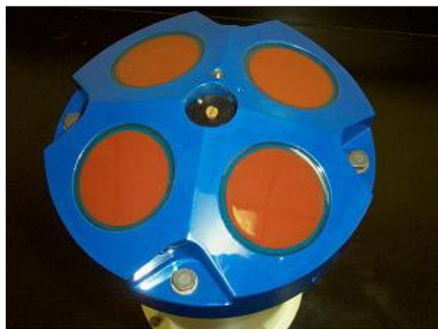
Figure 15. Image of a typical four-beam acoustic Doppler current profiler (ADCP) sensor head. The ADCP measures the speed and direction of ocean currents using the principle of “Doppler shift.” Photo courtesy of NOAA Ocean Explorer.
