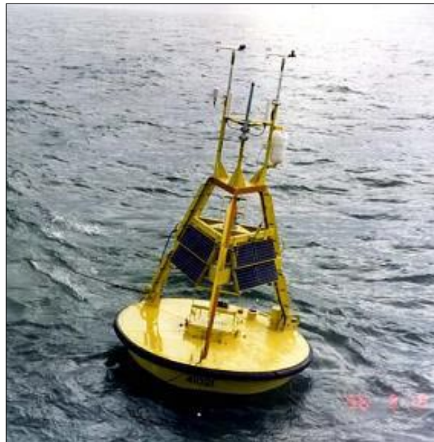
Figure 14. A three-meter NOAA buoy collects weather data by measuring wave height and period, as well as other weather parameters such as wind speed and direction. Photo courtesy of NOAA National Data Buoy Center.
