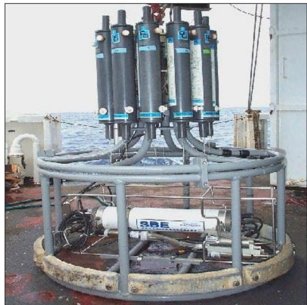
Figure 11. CTD instrument. Photo courtesy of NOAA National Marine Fisheries Service, Southwest Fisheries Science Center.
