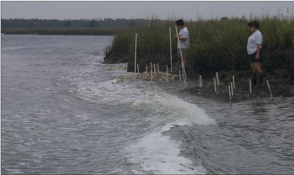
Figure 24. Small-scale experiments to assess the impact of boat wakes 9 on newly planted Gulf shell in Inlet Creek in April 2000. Photo courtesy of Loren Coen, Marine Resources Research Institute, South Carolina Department of Natural Resources.
