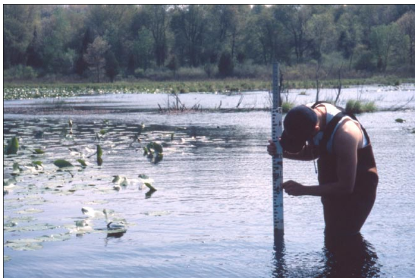
Figure 16. An extra length of gage is being added to this pole to measure higher water levels. Photo by David H. Merkey, NOAA Great Lakes Environmental Research Lab.
