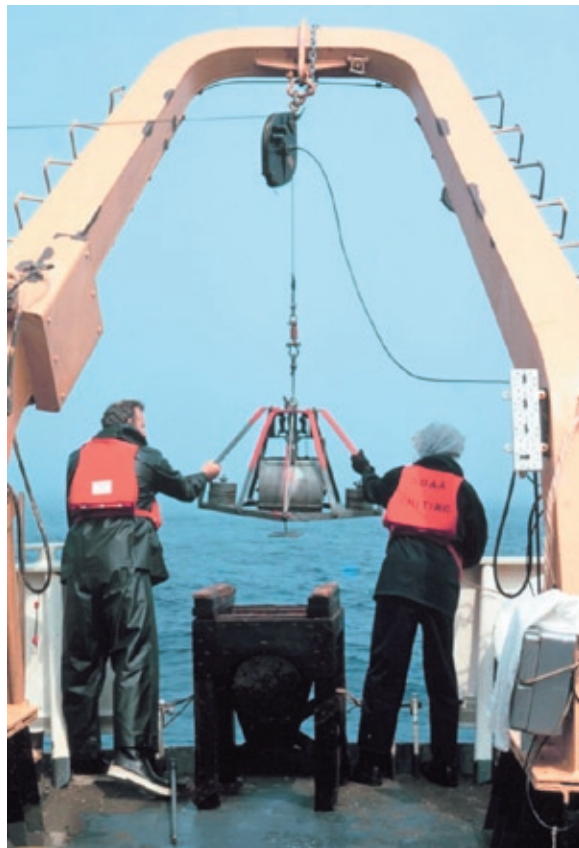
Figure 18. Grab sampler being used to determine soft bottom characteristics. Photo courtesy of Robert A. Pawlowski, NOAA Corps. Publication of the NOAA Central Library. http://www.photolib.noaa.gov/fish/fish1017.htm
