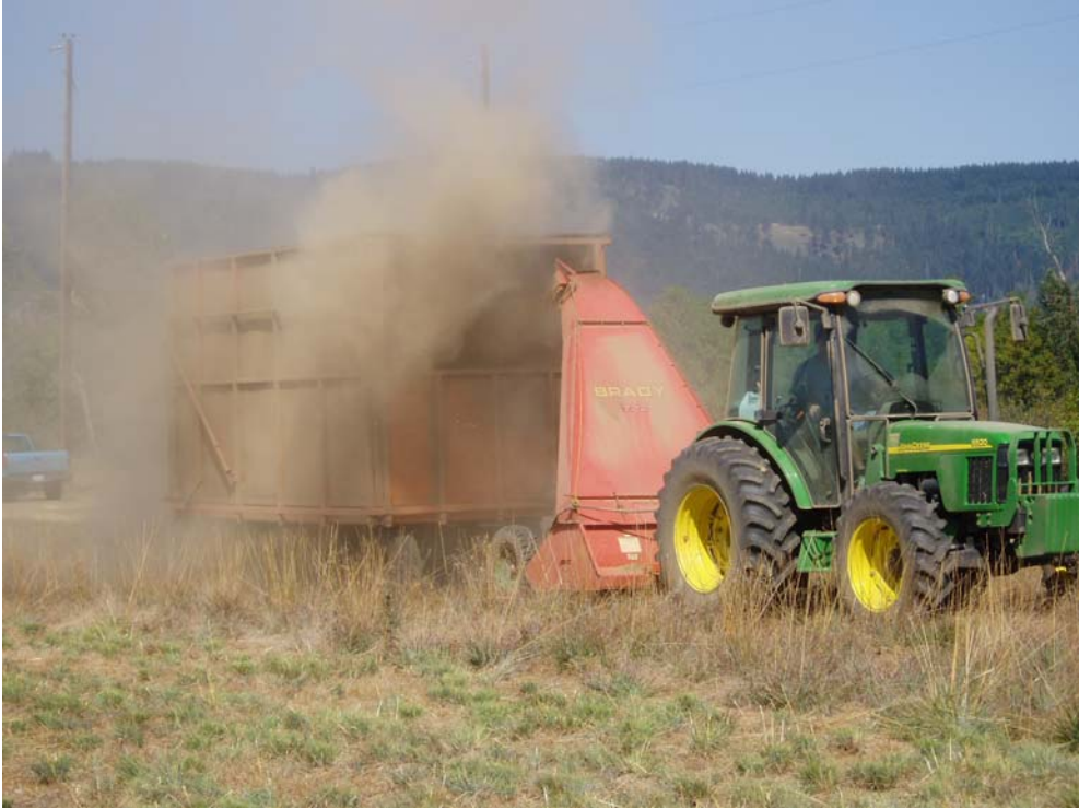
Figure 4. Brady flail chopper removing residue from seed increase fields.
