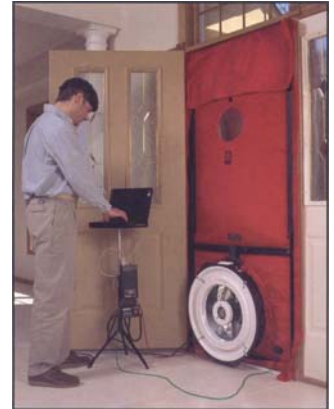
Home Energy Rater performs a blower door test.
