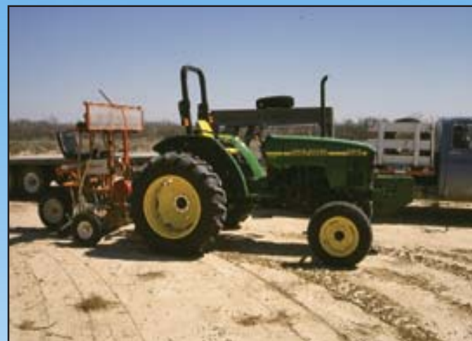
Plot drill used to seed varied grasses into brine test site
