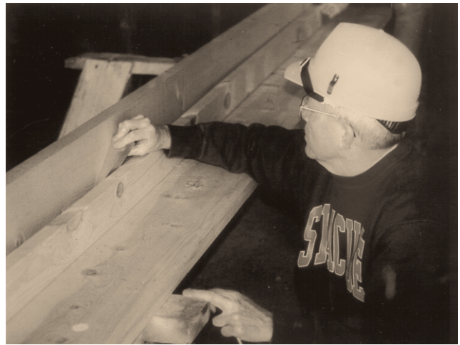
Figure 2—Measuring warp in ponderosa pine 2 by 4's from Arizona.
