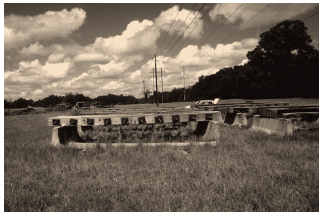
Figure 5—Test decks on concrete barriers.
