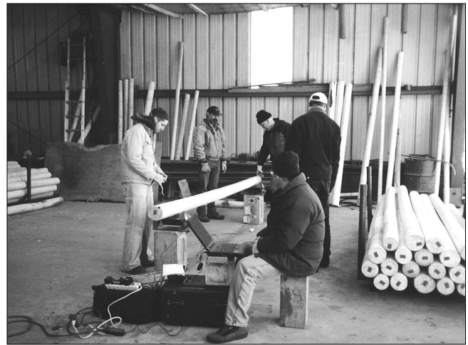
Figure 4. Determination of modulus of elasticity in transverse vibration of green lodgepole pine logs at Seeley Lake, Montana, using a prototype machine (photo courtesy of Karen Kovatch, the Intermountain Roundwood Association).
