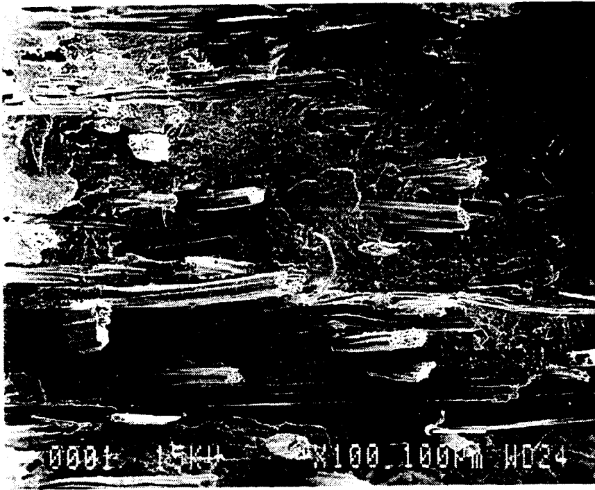
FIGURE 5. —Scanning electron micrograph of a jute fiber-reinforced polyester composite. Note the fibers pulled out of the matrix, which indicates poor adhesion of the matrix to the fiber.
