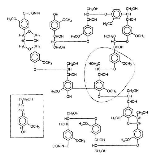
Fig. 2.1. Common structures of softwood lignin, with an example of the major arylglycerol-B-aryl ether structure circled. The inset shows coniferyl alcohol, the phenylpropanoid building block of softwood lignin.
