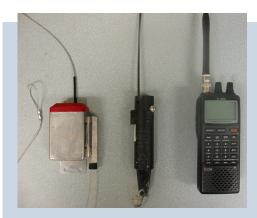
From left to right: a Telonics monitor, an ATS monitor, and an Icom receiver.
