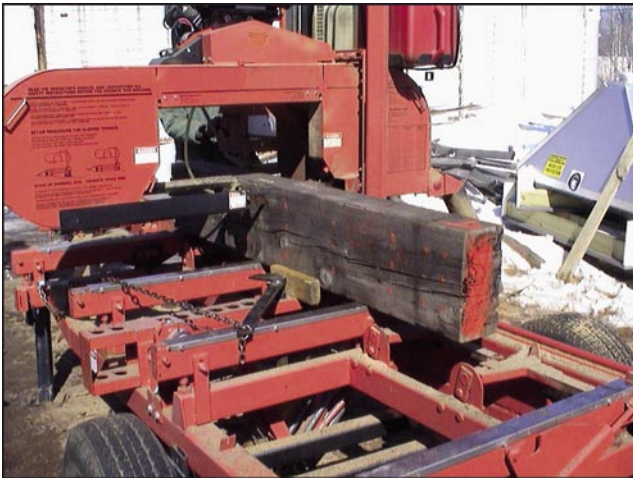
Figure 4—Portable band saw cutting timbers lengthwise along measurement lines.
