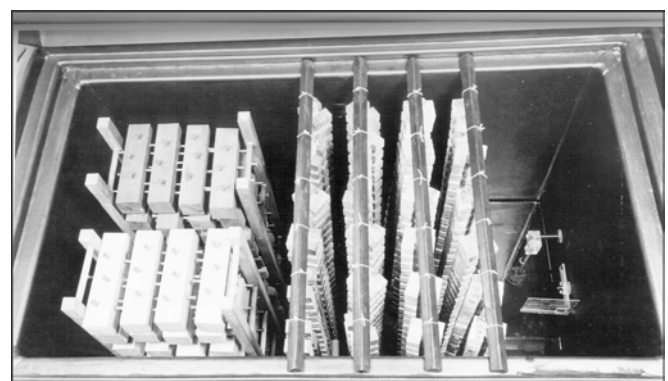
Figure 6—Salt-spray cabinet and specimens of Richolson (1959).
