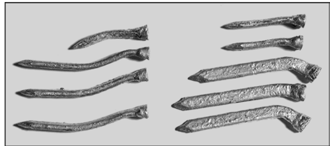
Figure 4—Mode IV (left) and mode III nail failures.
