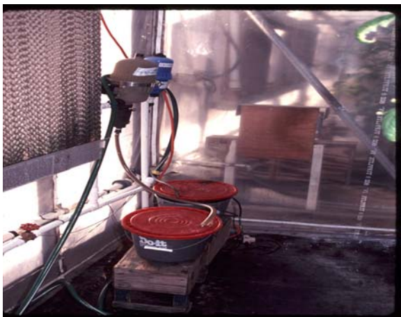
Photo 3. Drip irrigation system with Dosatro injectors and stock tanks.
