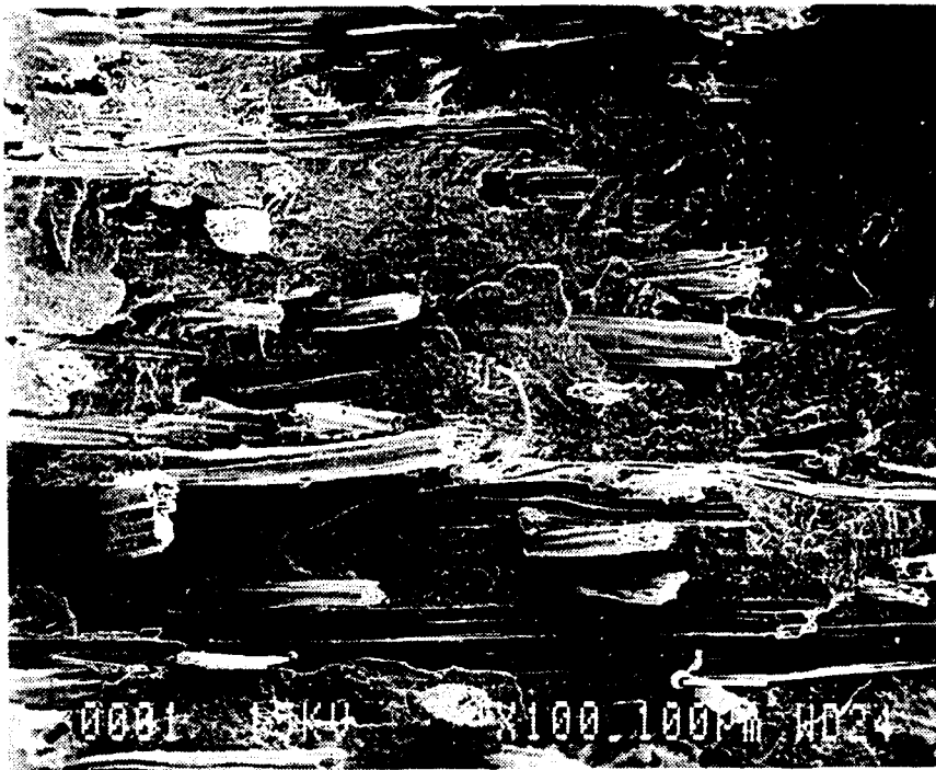
FIGURE 5. —Scanning electron micrograph of jute fiber-reinforced polyester composite. Note the fibers pulled out of the matrix, which indicates poor adhesion of the matrix to the fiber.
