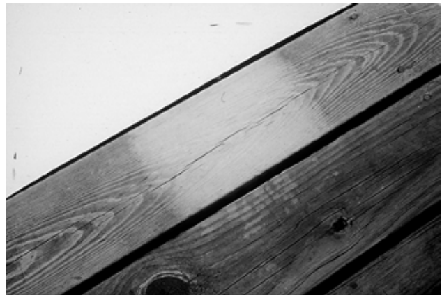
Figure 10—Growth of mildew on CCA-treated lumber. In cleaned section, mildew was removed with a bleach and water solution.
