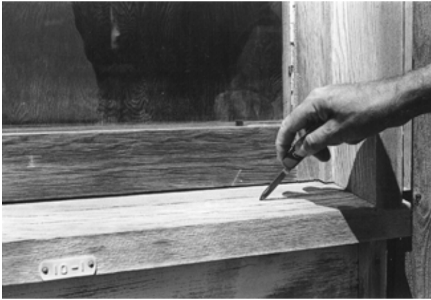
Figure 13—WRP-treated window unit after 20 years of outdoor exposure. The WRP-treated wood is firm and resists penetration by the knife blade.
