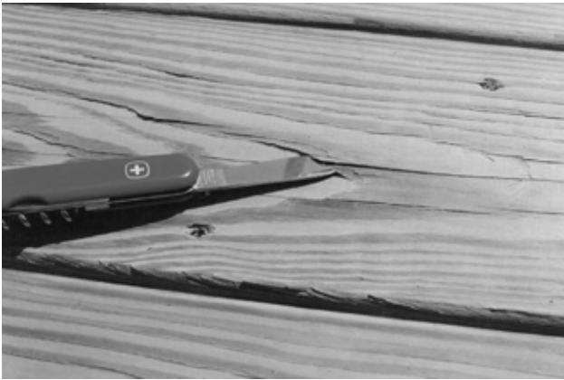
Figure 7—Raised grain on flat-grained lumber (tangential).
