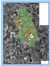
Figure 3: Aerial view map of 4,000 hectare watershed. Strata by drainage area: Orange: Strata 1 < 100 hectares Yellow: Strata 2 100-500 hectares Purple: Strata 3 500-1500 hectares Blue: Strata 4 > 1500 hectares
