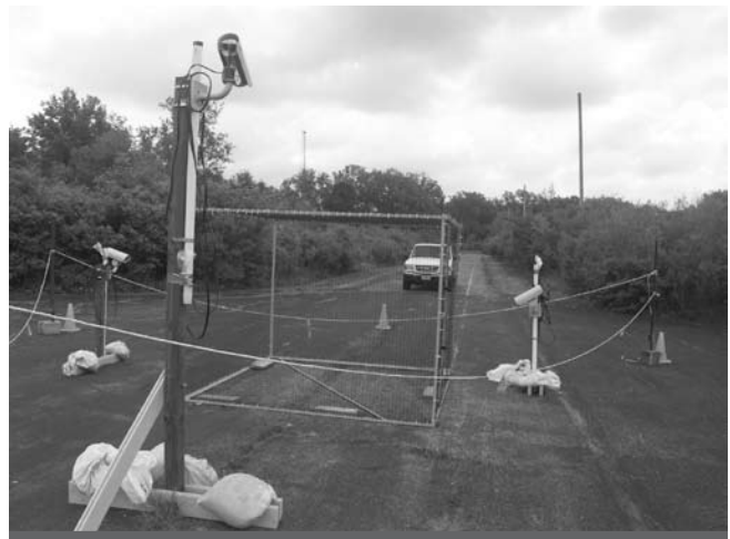
Three cameras are used to monitor the reaction of birds to the lighting system of an approaching vehicle. A fourth camera mounted on the vehicle monitors the birds' reactions from the perspective of the vehicle. The data from the four cameras are recorded simultaneously onto a digital video recorder for subsequent analysis. (APHIS photo by Robert Beason.)
