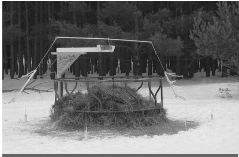
Frightening device for deterring deer from cattle feeders. (APHIS photo by Kirk VerCauteren.)
