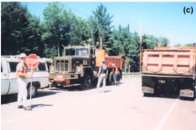
Figure 19—Truck positions for load test 2 for three load cases (looking north): (a) load case 3, (b) load case 4, (c) load case 6.
