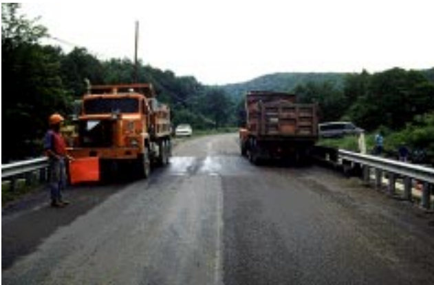
Figure 12—Truck positions for (top) load case 3 and (bottom) load case 6.
