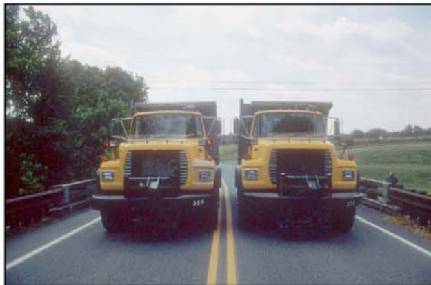
Millcross Road bridge: views of bridge, test sensor and load test.
