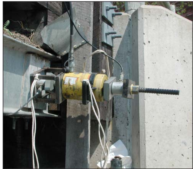
Figure 4—Hydraulic equipment and independent load cell used to check accuracy of monitoring load cell in measuring bar forces (Laurel Run bridge).
