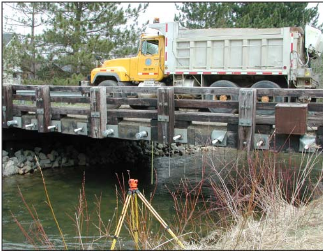
Figure 5—Typical setup for conducting static load tests with suspended rulers at midspan and an optical level instrument (Brookston Road bridge).
