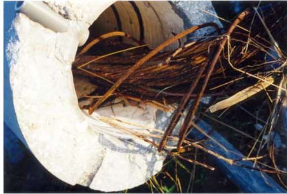
Figure 25. (a) Damage to hollow-spun concrete power poles at Carnation Road in Latte Heights, Dededo. (b) Some hollow-spun concrete power poles were improperly constructed with the pre-stressing steel cables bundled down the hollow center instead of being imbedded in the concrete. (NOAA Photos)
