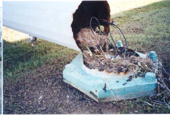
Figure 15. (a) Toppled bus in Tamuning. (b) Toppled light pole at the Paseo baseball field. Note thinness of the rusted metal at the base.
