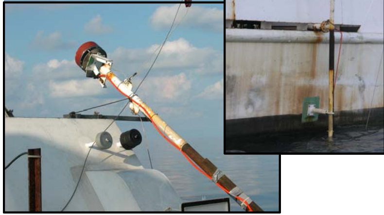
Figure 3. EM3000 Multibeam transducer secured using a mounting pole.
