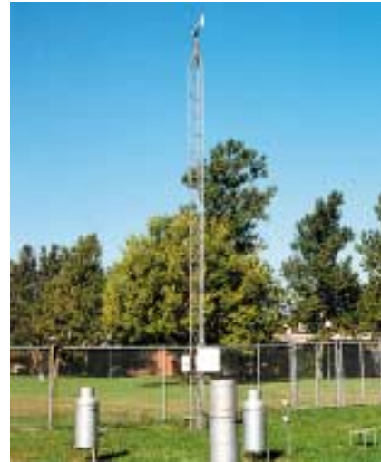
Instruments measure precipitation, wind, soil moisture, temperature, and humidity.
