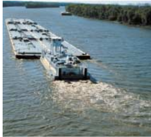
Barges on the Illinois, Mississippi, and Ohio Rivers require 9 feet of water when fully loaded.
