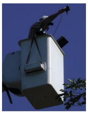
New remote-sensing technologies, such as hyperspectral imaging, hold great promise for quickly identifying areas of infestation of plant pests. A CPHST scientist is using a hyperspectral imaging device to validate data obtained from satellite imagery, a process known as "ground truthing."
