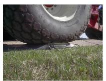
Figure 1. Weigh pad used to weigh a manure tank wagon.
