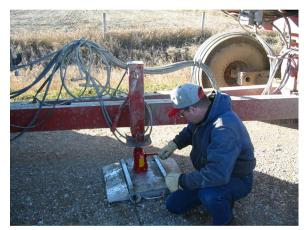
Figure 2. Weighing the hitch on a manure tank wagon.
