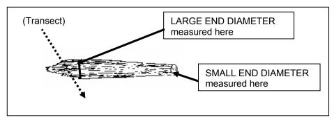
Figure 14-9. Example of decayed end intersecting the transect
