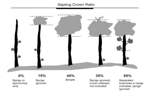
Figure 12-4. Sapling UNCOMPACTED LIVE CROWN RATIO determination examples.
